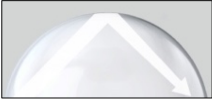
Figure 3. When an incident ray (lower left) reflects off a concave surface, it converges (becomes more focused).
