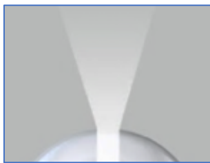
Figure 2. Since the surface of a sphere is concave, a ray of light diverges, or becomes less focused , after passing through a sphere. The more focused it is, the less it diverges. (Copyright held by the author.)
